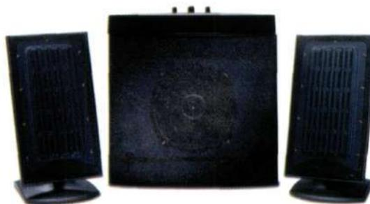
200 Hz third-order active crossover. The controls on the woofer enclosure adjust overall bass level, volume, and on/off 6 dB bass boost at 55 Hz. That's a lot of stuff for \$229 at retail, even if none of it qualifies as "audiophile" grade. Sonigistix's parts buyer must be quite resourceful. (Incidentally, the Monsoon MM-1000 is included in some Micron Millennium computer packages.)
