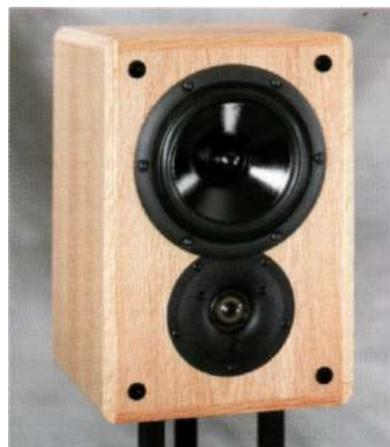
dome tweeter. The woofer, with composite paper cone (arguably still the best material for large diaphragms), phase plug, and polymer chassis, is mounted above the tweeter. The enclosure is vented to the rear. The silk dome of the tweeter is slightly recessed in a shallow hornlike cavity. The crossover network is second-order.
